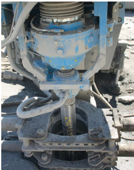
VD100 drilling in granite, 25 m deep, hole diameter 120 mm, flushing with air
