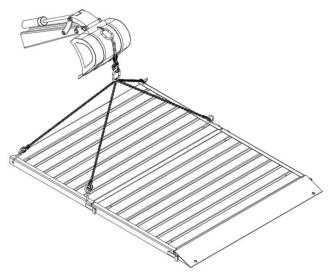
Move using suitable lifting gear and sling (min. 13 mm 4strand chain with a GS certification mark). The chain hanger to be provided by the customer is to be secured to the four suspension bolts on the top of the panel.
