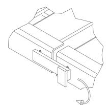
To secure the locking bolts, turn them 180°. The long end of the locking bolt must be vertical and facing downwards.
