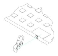
Laying is carried out using suitable lifting gear and slings (4-strand chain with GS approval).
