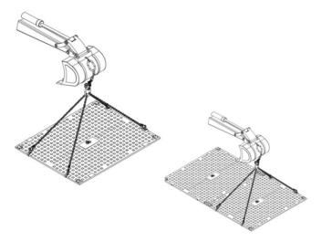
The site road panel can now be positioned. For this purpose, it should be moved as close to the ground as possible, in a horizontal position. Make sure that no persons are in the danger zone or swivel area.
