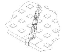
Then the load hooks of the chain sling must be hooked into the suspension rings of the sling gear. The closed position of the safety latch must be checked.
