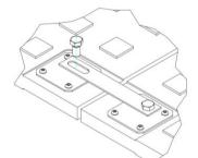
The panels are connected by means of metal connectors and hexagon head screws. First the metal connector is connected to the panel in the circular hole by a screw. Then the screw is mounted in the slotted hole.
