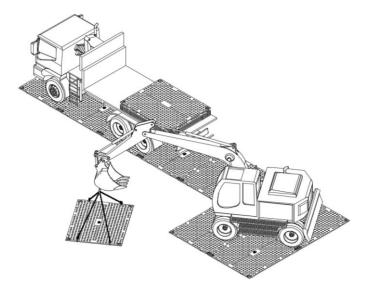
The site road panels can be laid continuously and can be passed over after fixing. Passing over with crawler type vehicles is only permitted with rubber tracks and requires prior instruction.
