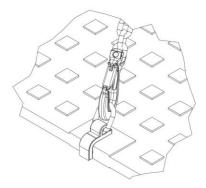
Then the load hooks of the chain sling must be hooked into the suspension rings of the sling gear.
