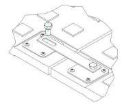
The panels are connected by means of metal connectors and hexagon head screws. First the metal connector is connected to the panel in the circular hole by a screw. Then the screw is mounted in the slotted hole.
