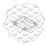
If the panels are laid over a larger area, the panels are fastened to each other in a clockwise sequence.
