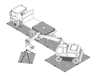
The site road panels can be laid continuously and can be passed over after fixing. Passing over with crawler type vehicles is only permitted with rubber tracks and requires prior instruction.
