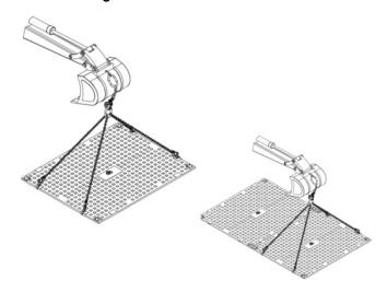
The site road panel can now be positioned. For this purpose, it should be moved as close to the ground as possible, in a horizontal position. Make sure that no persons are in the danger zone or swivel area.
